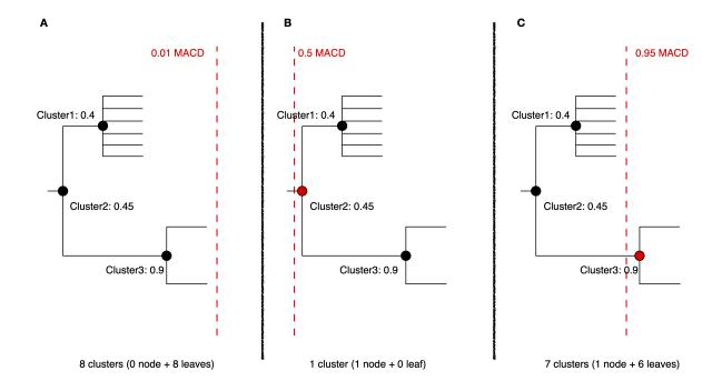
In Figure A, a very small cutoff value results in no nodes being selected, leaving a set of 8 clusters or singletons. When the cutoff is increased to 0.5 in Figure B, only one cluster, Cluster2, is selected. However, when a higher cutoff value of 0.95 is adopted, Cluster3 is selected, and the remaining six isolates are left as singletons, resulting in a total of 7 clusters.
