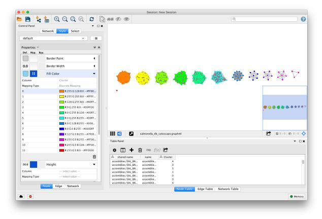
In some cases, edges which are between strain links may have been erroneously included in the network. This could be due to poor model fit, or a poor quality sequence. Use Tools -> NetworkAnalyzer -> Analyze Network to compute information for each node and edge. It may help to analyze connected components separately. They can be split under Tools -> NetworkAnalyzer -> Subnetwork Creation.
